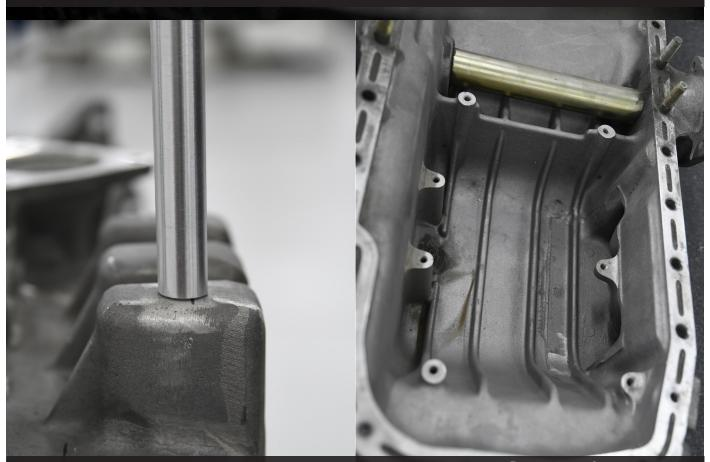
When placing the tubes into the sump prior to welding, the flat side of the tubes should sit on the strengthening ribs in the bottom of the sump to ensure that they can scavenge the maximum amount of oil at the lowest part of the sump.
